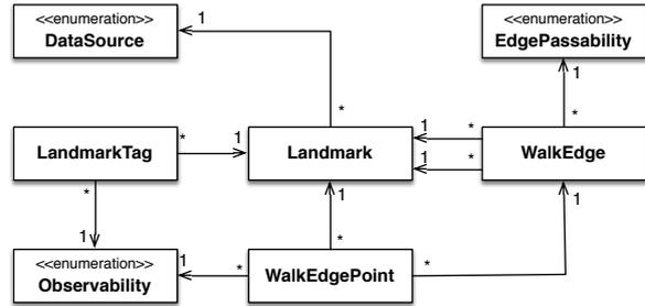
**Fig. 1.** Diagram of the primary database entities that are used to store and update data from multiple sources.
