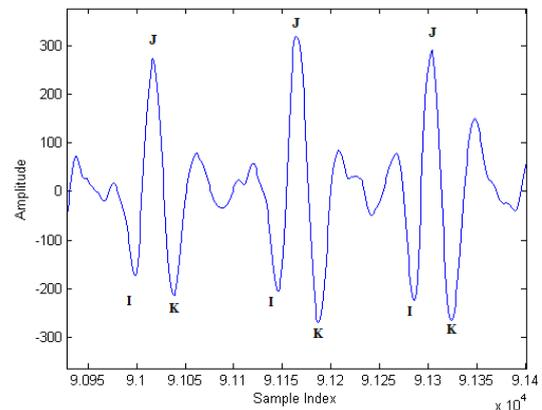
Fig. 1: Typical BCG waveform showing I, J, K points.
