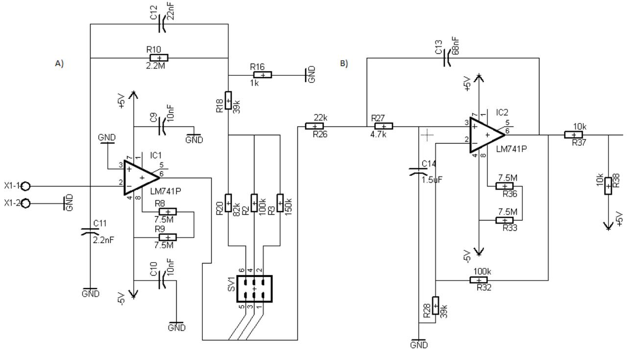
Fig. 4: Signal conditioning circuit. A) charge amplifier stage with selectable gains, B) low pass filter stage.
