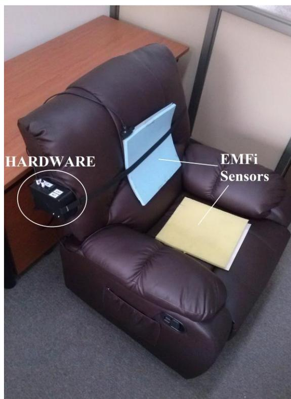
Fig. 7: System set-up in a couch. EMFi sensors are 30 cm x 30 cm and covered in foam for protection.
