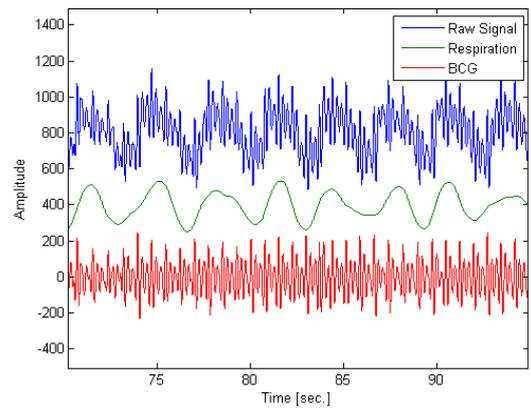
Fig. 5: Wavelet signal processing, the respiration signal correspond to the approximation of the original signal, and the BCG correspond to the details.
