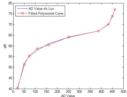
Fig. 3: Polynomial relation between AD conversion and sound intensity (dB).
