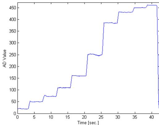
Fig. 2: Sound sensor output during sound test using 800 Hz tone and different intensities.
