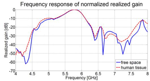
Fig. 4: Simulated frequency responses of normalized realized gain of the filtering antenna in free space (solid blue line) and on human tissue (dashed red line).
