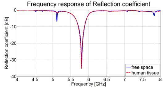
Fig. 3: Simulated frequency responses of reflection coefficient at the input of filtering antenna in free space (solid blue line) and on human tissue (dashed red line).
