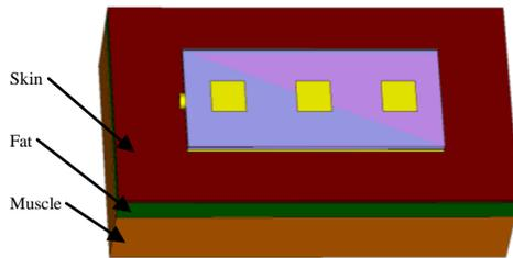
Fig. 2: Filtering antenna on a model of human tissue.
