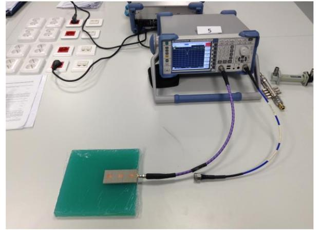
Fig. 8: Measurement setup for the characterization of the filtering array on the phantom.
