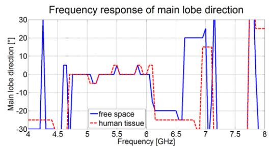
Fig. 5: Simulated frequency response of the main lobe direction of the filtering antenna in free space (solid blue line) and on human tissue (dashed red line).
