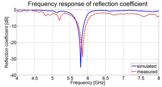
Fig. 7: Frequency response of reflection coefficient at the input of the filtering antenna on the phantom: simulation (solid blue line) versus measurement (dashed red line).
