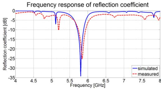
Fig. 6: Frequency response of reflection coefficient at the input of the filtering antenna in free space: simulation (solid blue line) versus measurement (dashed red line).
