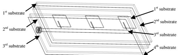
Fig. 1: Structure of three-element filtering antenna array fed by apertures.
